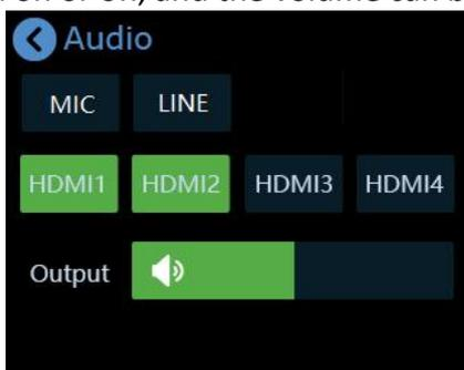
The audio input can be selected as MIC passive microphone input, or LINE input audio console or active microphone signal input according to needs.
