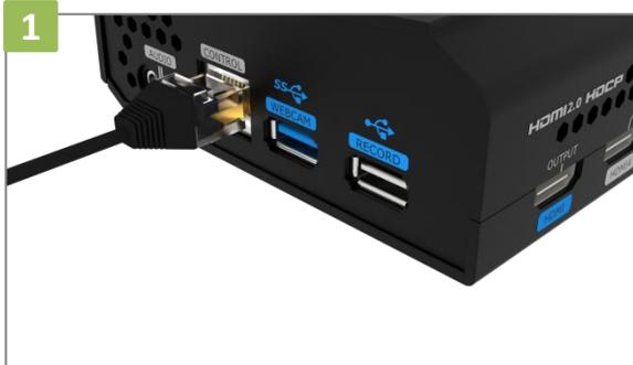
1. Connect the mini-pro to the router's LAN port.
