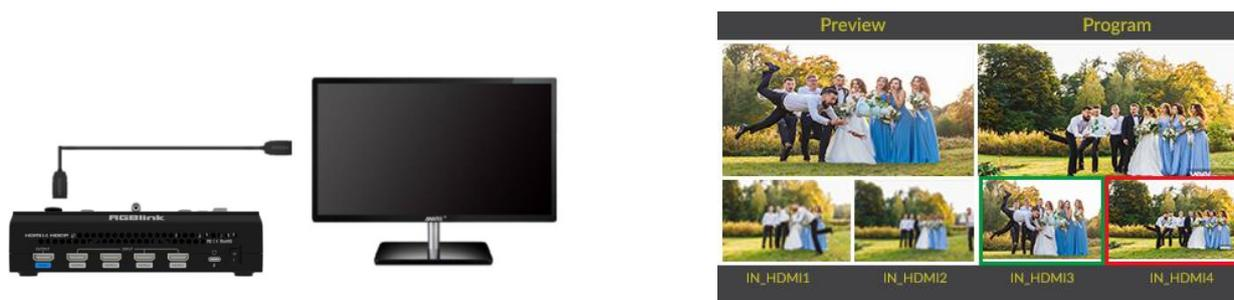
In addition to supporting multi-screen monitoring, HDMI output also supports single screen display of any one of the four inputs. You can switch between PVW and PGM In **【Video Output】** menu.
