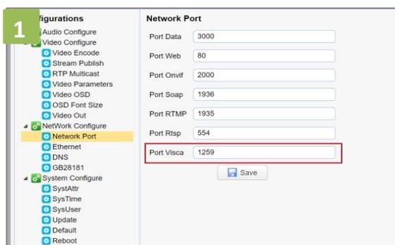
1. Set the corresponding communication port on the PTZ camera, such as VISCA or UDP port 1259.
