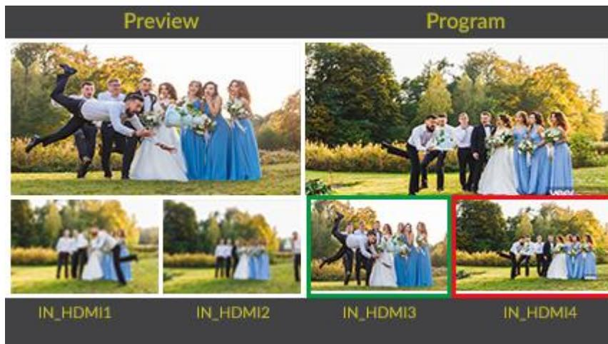
The **【LCD Info】** is LCD display setting, which controls whether the 2x2 video preview is **【simple】** or as **【standard(PVW)】**, turn on **【LCD Info】** to check the resolution of four inputs as shown in the picture below:
