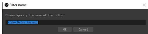
5. Input delay value in ms, the value need to adjusted until the video and audio is synchronous.
