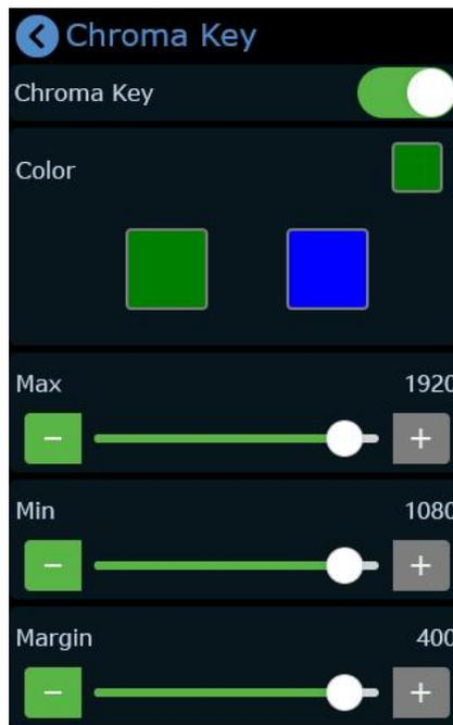
(4) After the Chroma Key is set, the parameters can be saved directly on the device. Next time when the the device is on no matter on the dominant software XPOSE mini or the touch screen itself, users can directly load the preset. And the layer selection stays at main screen, that is, directly press the signal key, the main screen is switched.
