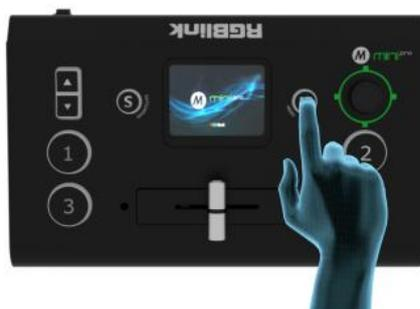
As shown in the figure below, the UI style on the touch screen is similar to current smart phone operating interface. The first-level menu is in icon. You can quickly enter the corresponding function management interface by tapping the corresponding icon.
