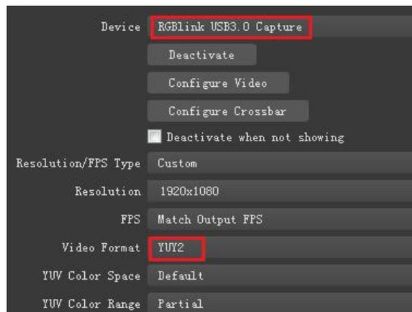
**Note:** If there is no video format YUY 2 after setting above, check the USB 3.0 port connection. Make sure it is linked to USB 3.0 port on PC by USB 3.0 cable. (USB 3.0 cable or port is standard in blue while USB 2.0 is in black). If the captured, change the video format to YUY2.
