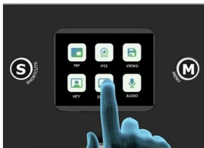
You can enter the **【Effects】** selection interface, where fade in, fade out and various other transition effects can be selected. The inside icons on the menu can be dragged and sorted according to your preferences. When the selection is completed, the root directory icon will be replaced with the last selected icon.
