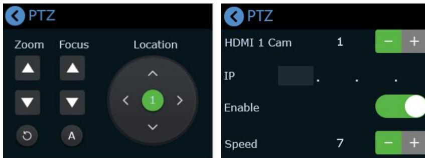
When setting PTZ, use the signal key ①②③④ to select the corresponding PTZ camera signal to preview.
