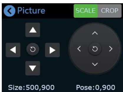
In addition to adjustment by moving the slide rail, you can also use the toggle to quickly adjust the size of the sub-picture, and use the joystick to quickly adjust the position of the sub screen. If you need to quickly switch to the PGM, you can press the joystick.
