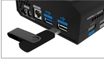
mini-pro will automatically recognize the hard disk or U disk and display the relevant information on the recording window of multi-screen PVW .
