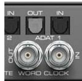
Selecting *Single Speed* in the Settings dialog causes the output signal to always stay within the range of 32 kHz to 48 kHz. So at 96 kHz and 192 kHz sample rate, the output word clock is 48 kHz.
