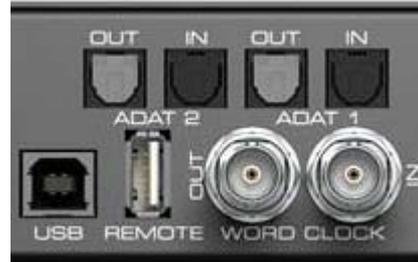
**ADAT2 I/O.** TOSLINK. Standard ADAT optical port, 8 channels. Can also be used as optical SPDIF input and output, if set up accordingly in the Settings dialog.
