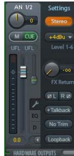
**Loopback.** Sends the output data to the driver as record data. The corresponding submix can be recorded then. This channel's hardware input sends its data only to TotalMix, no longer to the recording software.
