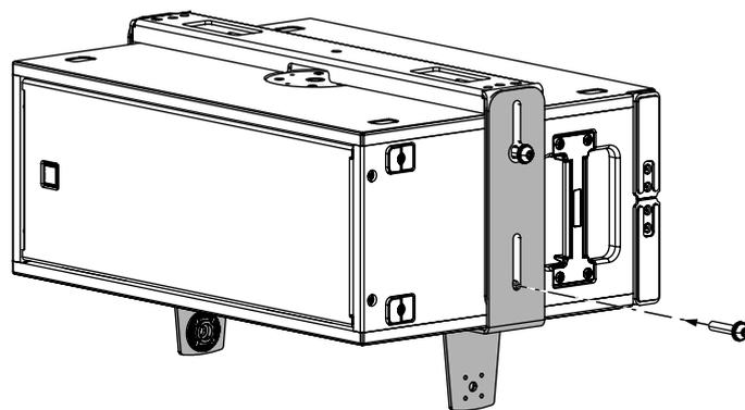
3. Pull down the bracket and tighten both the upper and lower screw.
