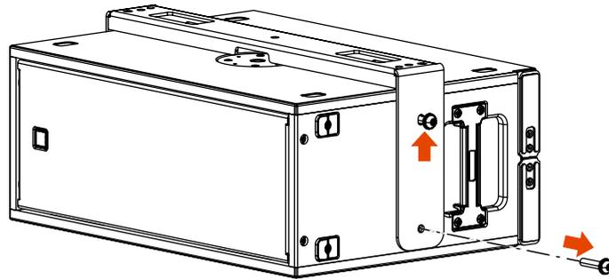
2. Place the link bars on both sides and letting the upper screw pass through the circular bottomhole; then screw back the lower screw (do not tighten the screw yet).
