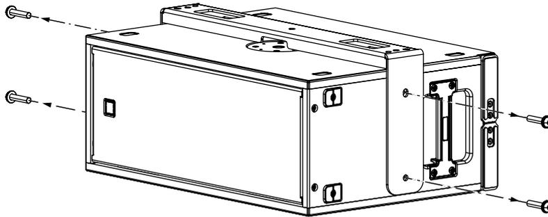
2. Place the linking brackets on both sides (as shown in the picture) and screw them to the cabinet with the same M10 screws (and washers) removed earlier.
