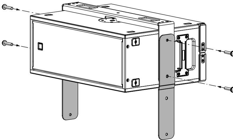
3. Place the second subwoofer in cardioid configuration and screw the bracket to it with the M10 screws provided.
