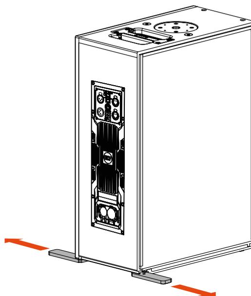
When used on vertical position, slide the two plastic plates on the bottom of the speaker for a better stability and safety.
