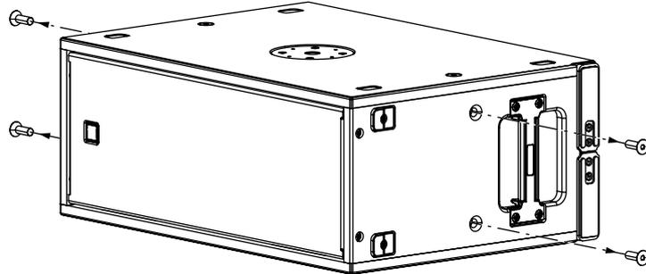
2. Place the bracket over the speaker and screw it to the cabinet with the four M10 screws (and washers) provided.
