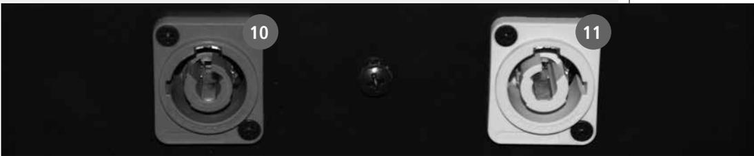
10 AC INPUT. Powercon locking 3-pole AC mains.
