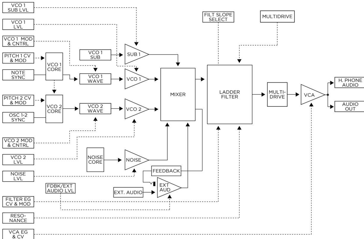
You can control the Subsequent 37 using control voltages and MIDI commands. When the Subsequent 37 receives either a control signal from the onboard keyboard or a Note On command from an external MIDI source, it responds by sending a gate signal to trigger the envelopes and a control voltage (CV) to control oscillator pitch. The envelopes respond by sending control signals to the amplifier and filter.
