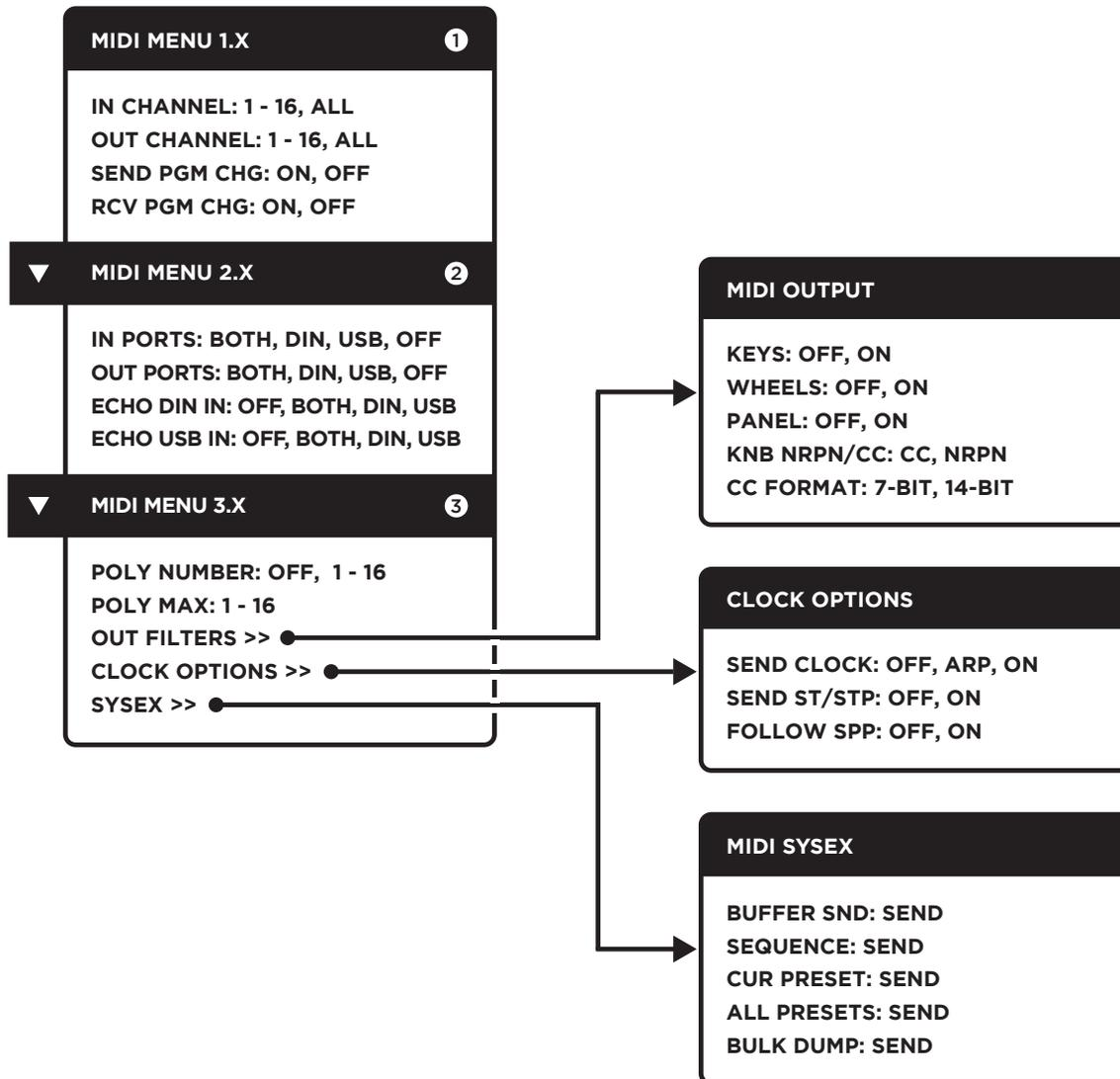
Press the **MIDI** button to open the **MIDI MENU**. This menu contains parameters associated with the sending and receiving of MIDI signals. When the **MIDI** button is illuminated the top right of the LED display will indicate which page you are on, followed by a decimal point, and then which parameter line you currently have selected. Use the ▼ ▲ buttons to choose a parameter for editing, and the **FINE TUNE** knob to scroll through a selected parameter's available options.
