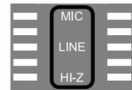
The MIC (XLR) or LINE (1/4") combo inputs on the rear panel are selected by the pressing the INPUT button when the channel is selected. The HI-Z input (available on channels 1 and 2 only) is selected automatically when an instrument cable is plugged into a Hi-Z input on the front panel.
