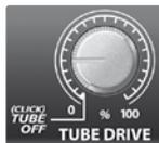
**Tube Drive.** Tube Drive controls volume being routed through the 12AX7 vacuum tube, unlike the Input Gain which controls the overall volume. The effect achieved ranges from subtle to extreme, depending on the setting being used. The more signal being sent to the tube, the more distortion you will hear. While you won't always want to use tube drive, it can be a great choice for guitar, bass, and even vocals.
