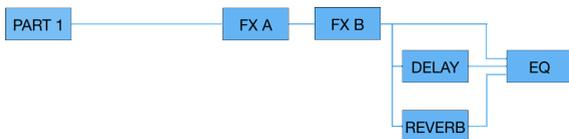
Part 1 hosts the Instrument, which feeds two insert Effects (FX-A and FX-B) routed in series. This means that the output of FX-A feeds the input of FX-B. The output of FX-B can then be sent independently to the Delay and Reverb effects. The outputs of FX-A and B, the Delay, and the Reverb then all feed the 3-band master EQ, the final output of which is controlled by AstroLab's master volume knob.
