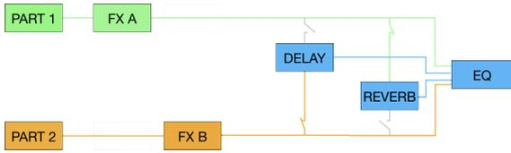
Parts 1 and 2 and their respective Instruments feed one insert effect or the other. The output of each insert effect can then be sent to the delay, reverb, or both. Four outputs are summed into the master EQ: Part 1 and its insert effect (pre delay and reverb), Part 2 and its insert effect (pre delay and reverb), Delay output, and Reverb output.
