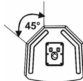
The rear side inclination, symmetrical, as shown in the upper picture, is 45°. KL10 can be used as a stage monitor in small contexts, in this case please consider the characteristic dispersion pattern presented above.
