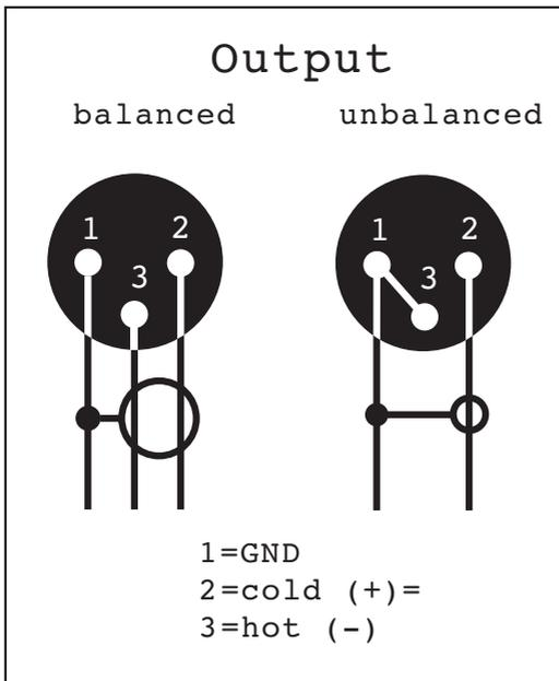
unbalanced signals to the balanced XLR connectors:
