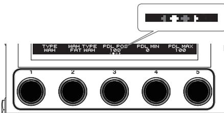
Use the PAGE [◀] [▶] buttons to switch between the parameters that you want to edit. The current page is indicated in the lower center of the screen.
