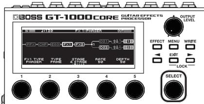
The selected block is enclosed by a thick frame.
