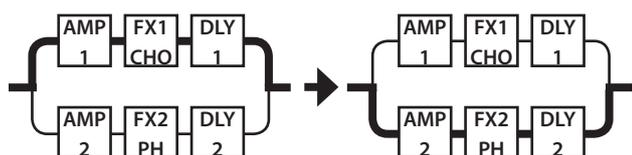
The same chain is used for both patches, both before and after switching. The settings of the effect used before switching are placed in parallel with the settings used after switching.
