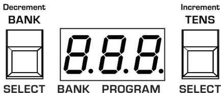
Use the Bank and Tens buttons to scroll forward and backward, respectively, through parameter settings
