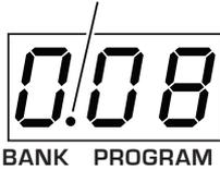
The dot illuminates when a knob position matches a preset's saved parameter value
