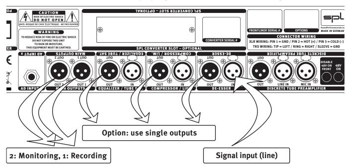
This example shows the exclusion of de-esser, compressor and EQ/tube saturation as a group. The input signal is connected to the input of the first module. If all three processors are excluded as a group, the output signal of the group is present at the MAIN OUTPUTS. If a dual processor group is excluded, the output of the last module is always the group output. In the example above the preamplifier can be used separately via its own I/Os. Further information on page 25.
