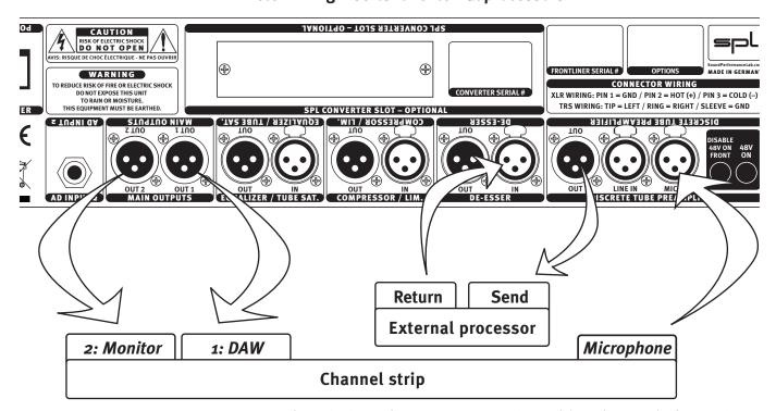
You can determine inserts between every processing module. In the example above, an insert is determined between preamplifier and de-esser. The insert is routed via preamplifier output and de-esser input as send and return. Refer to page 26 for further information.
