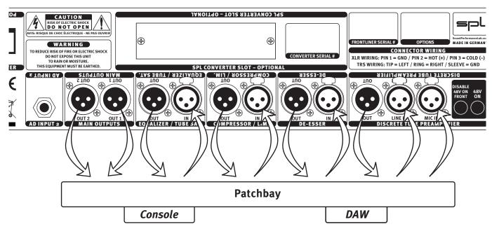
Our recommendation for studio wiring: all inputs and outputs are connected to a patchbay so that each Frontliner module can be routed with maximum flexibility within a studio environment. Connections to a console or to DAW interfaces for example can always be configured to meet the respective requirements. Aside from the switching options that the Frontliner provides the sequence of modules can be determined in any way with the patchbay.
