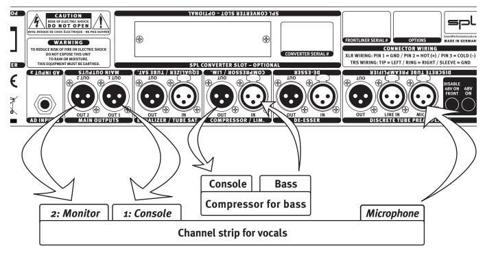
An example for a live setup: The compressor module is separated from the channel strip. The vocal signal can be processed with all remaining modules, while the compressor is used for processing bass. In the same way, each module can be taken out of the channel strip, e. g. using the De-Esser separately while processing an acoustic guitar with the (remaining) channel strip and so on. Detailed information on page 25.
