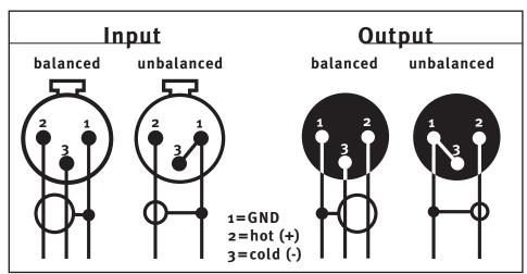
Connections to RCA sockets are always unbalanced, a wiring to jack connectors can be both balanced (1/4" TRS/stereo jack) or unbalanced (1/4" TS/mono jack). We recommend to use individually configured cables from XLR to RCA or jack sockets instead of adaptors. You can get cables in any needed configuration from audio dealers. With the diagram above, the dealer can ensure to provide the appropriate cable for your application.
