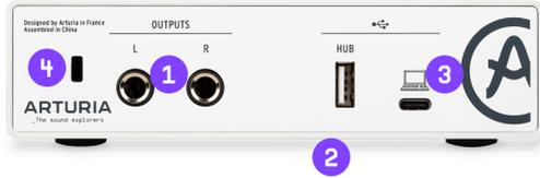
1. Outputs - these 1/4" balanced stereo outputs can be connected directly to active studio speakers or other devices such as amplifiers and mixers.
