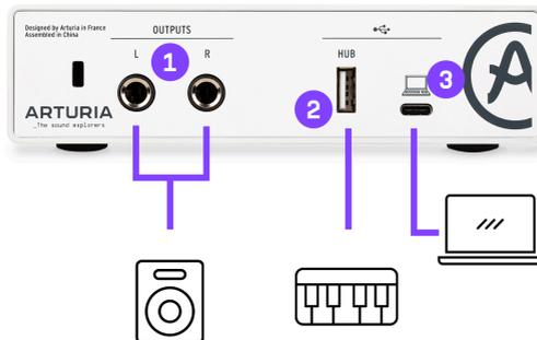
1 : TRS outputs to connect powered speakers or mixer/amplifiers
