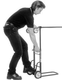
Loosen wingbolts 1/4 turn. Step on rear axle and push in extension stop button. Pull up on frame as shown until stop button engages. Retighten wingbolts.
