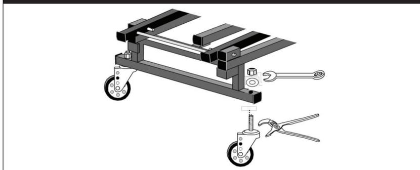
Attach front swivel casters as shown. While tightening lock nuts, grip bearing cap with channel lock pliers or pipe wrench to prevent threaded stem from turning. Tighten lock nuts firmly, but not excessively tight. Check lock nut tightness on caster stems periodically.
