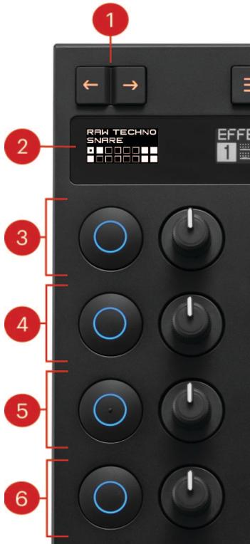
1. **Deck Assign Buttons:** Assign the Pattern Player loaded in this FX unit to a deck by pressing the arrow buttons. When the Pattern Player is assigned to a deck, the arrow button will light up in bright orange and stay lit. To remove the assignment simply press the button again. Traktor Pro treats the Pattern Player like any other FX unit, meaning assigning it to a deck does not replace the deck itself but rather plays on top of it.
