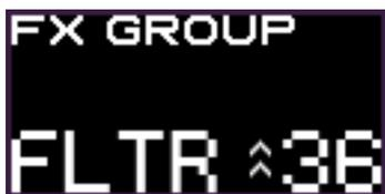
*The display of an FX unit indicating that a knob needs to be turned clockwise to start manipulating the loaded filter.*
