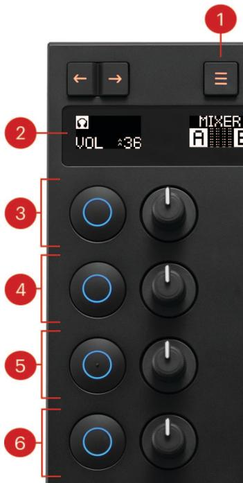
1. **Mode Select Button:** Press this button to enter mixer mode. If four FX units are configured in your layout you might have to press this button repeatedly until the central Mode display at the top shows MIXER.
