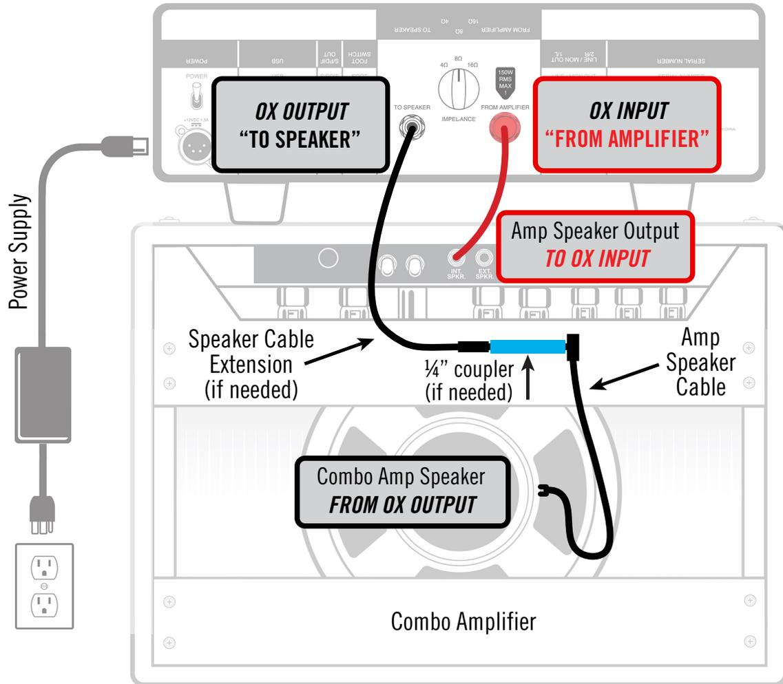
*OX high-power connections with a combo amp
