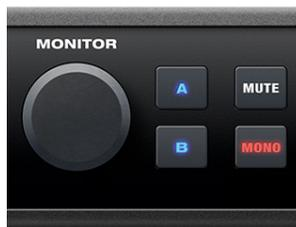
Figure 7-6: The front-panel monitor controls.
