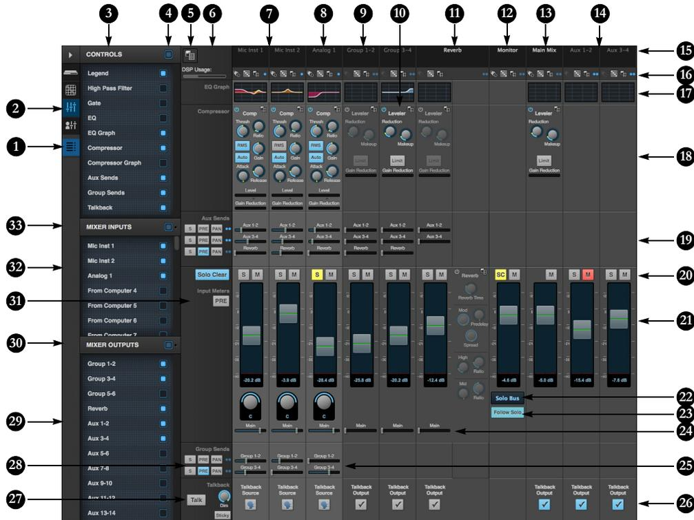
The Mixing tab gives you full access to the 48-channel mixer in the 828Es, which provides a main mix bus, monitor bus, three group buses, seven aux buses, and a dedicated reverb bus. Use the Device tab to configure how many inputs you wish to work with (up to 48). Use the Routing tab (page 15) to route channels to the mixer inputs. Channels can come from any source, such as the physical inputs on the interface, channels coming from the computer, or channels coming from the AVB network.
