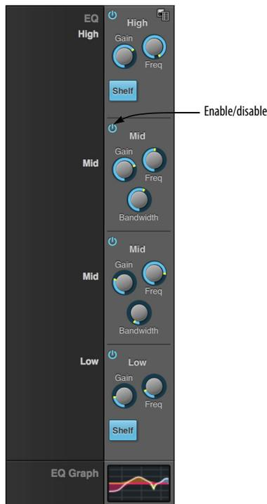
Figure 9-3: The Four-band parametric EQ module.
