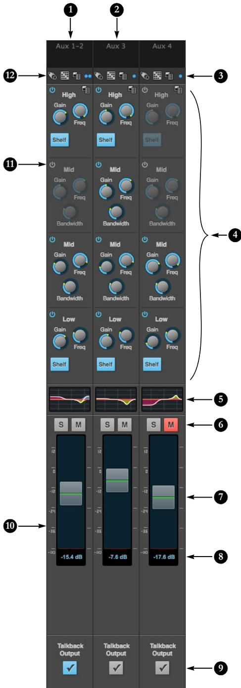
Aux buses can be used to create sub-mixes. An aux bus can be assigned to any output in the Routing grid (page 15).
