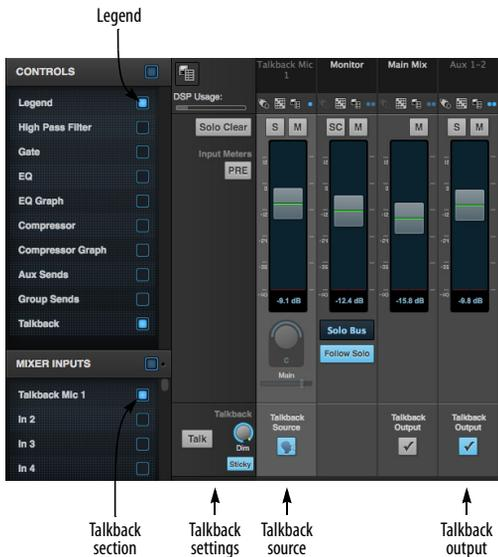
Figure 7-8: Mixer setup for the talkback mic.
